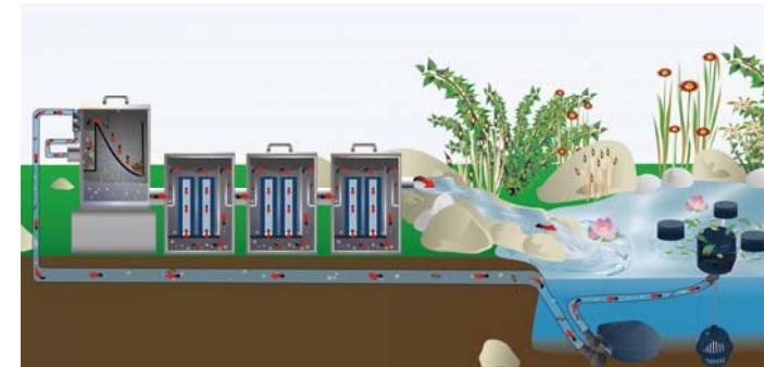
The filter system can be placed above pond water level. Through a pump (or a levelled FIAP Pump Active) dirty pond water is transported into the filter system. The already cleaned water runs back into the pond over a tube with a decline.
