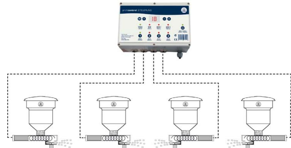
The buttons on the controller can FIAP proficontrol Control the running time in seconds (1 - 99). Wait time in minutes (1 - 99) and the motor speed can be adjusted in 99 steps for each output. The total FIAP proficontrol can be via a separate button on or off. The settings are retained after a reset (power off) is obtained.
